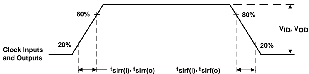
Figure 8. Input and Output Slew Rates
